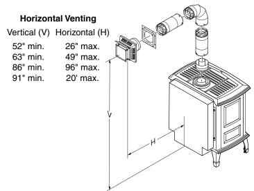
Figure 28 - Horizontal Termination Configuration for Venting Using One 90° Elbow
